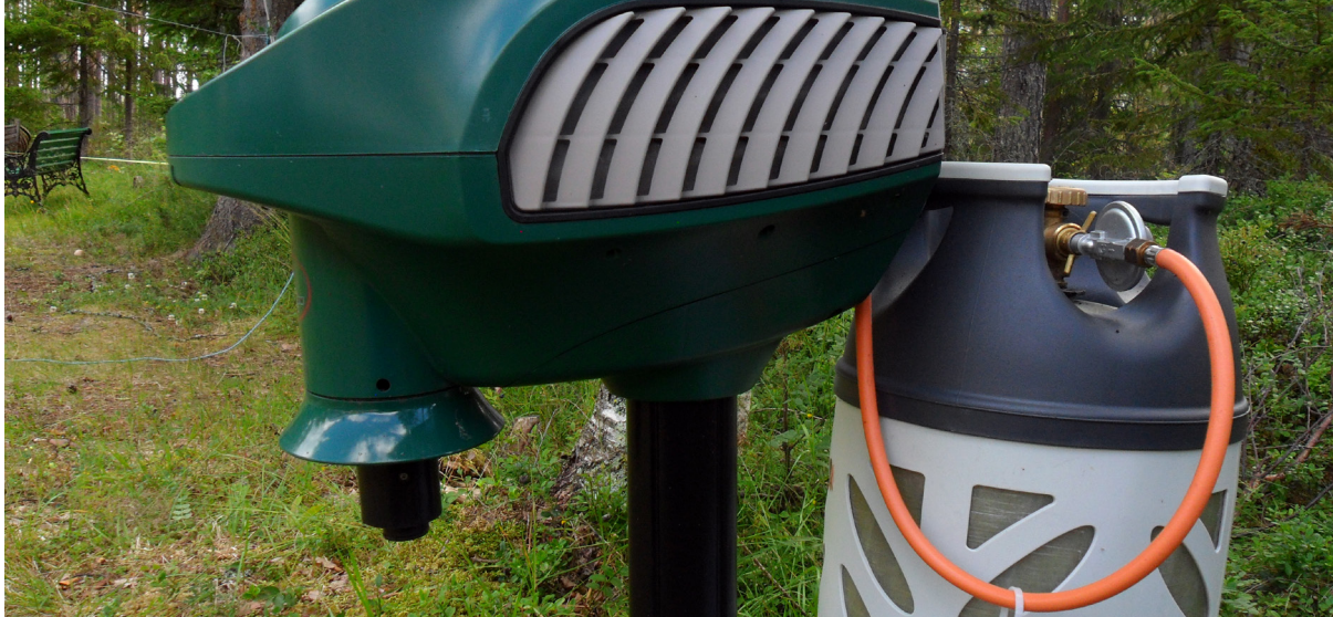
Powered by propane gas, this mosquito trap emits a plume of CO 2 , heat and moisture to attract and trap mosquitoes
