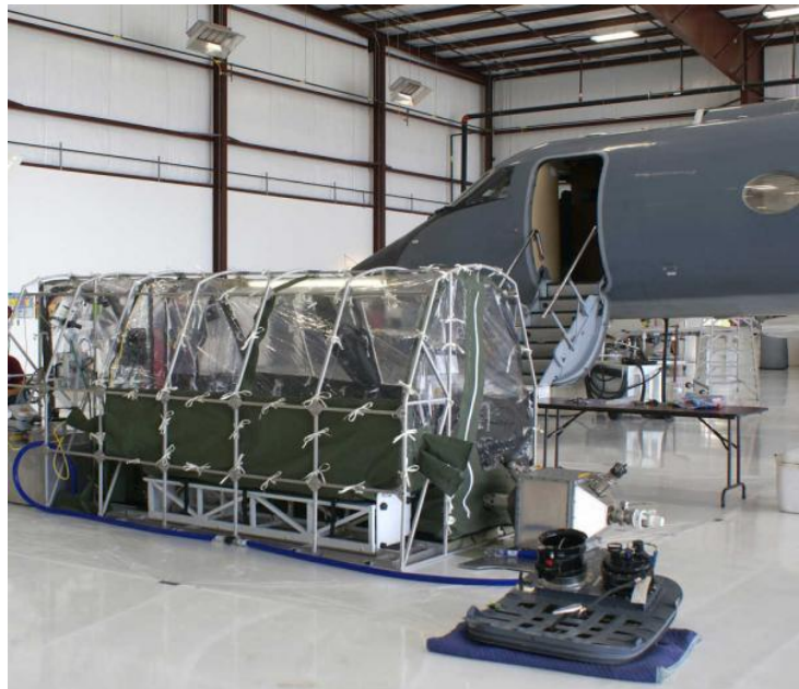
Aeromedical Biological Containment System, usually mounted inside the aircraft
